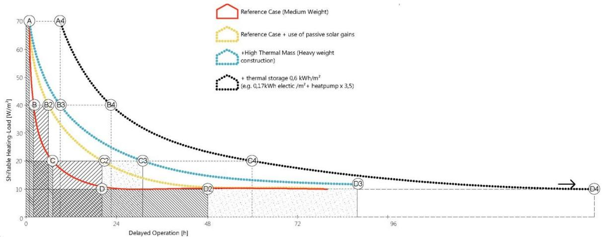
Fig. 3: Load duration curves of four different Austrian typology-buildings showing the potential of shiftable domestic heating load over time by delayed operation (Weiss et al. 2018)
