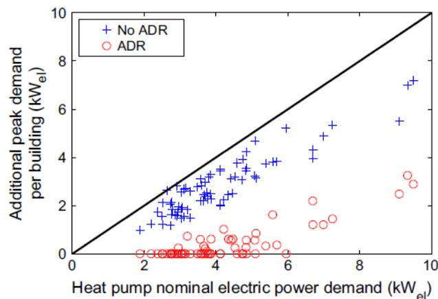
Fig. 2: Performance of ADR in peak-shaving. The electric power that each building is contributing to the demand at peak time is shown with respect to the nominal electric power demand of the heat pump (Patteeuw et al. 2015).
