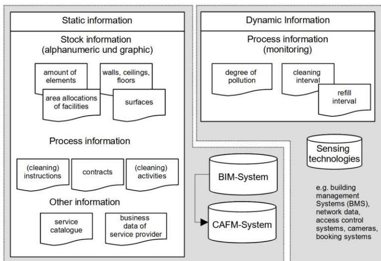
Fig. 2: Static and dynamic data for provision of services in FM
